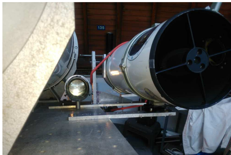
Platine mobile supportant un Newton 200/800
